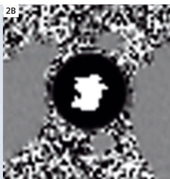
2 (A) Magnitude image of water flowing through a pipe, with (B) its velocity or phase image showing aliasing due to the VENC being set too low. The peripheral slower moving water is correct, but once the velocity reaches and then exceeds the VENC, there is an abrupt transition from black to white where the velocities are no longer correct.
