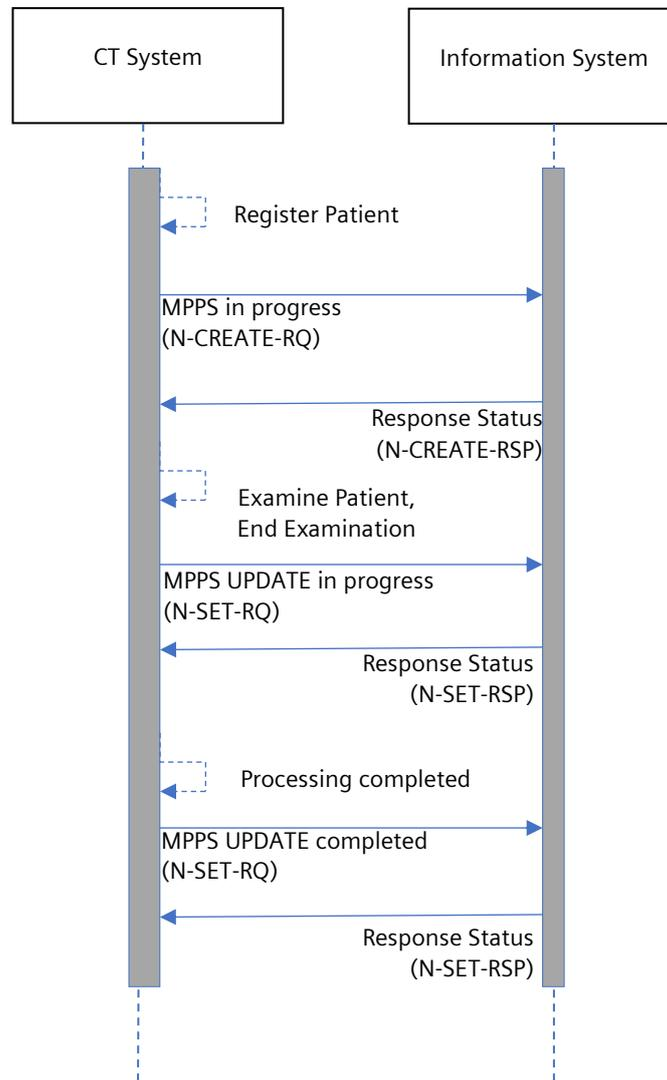
Figure 7: Sequence Diagram – Modality Performed Procedure Step
