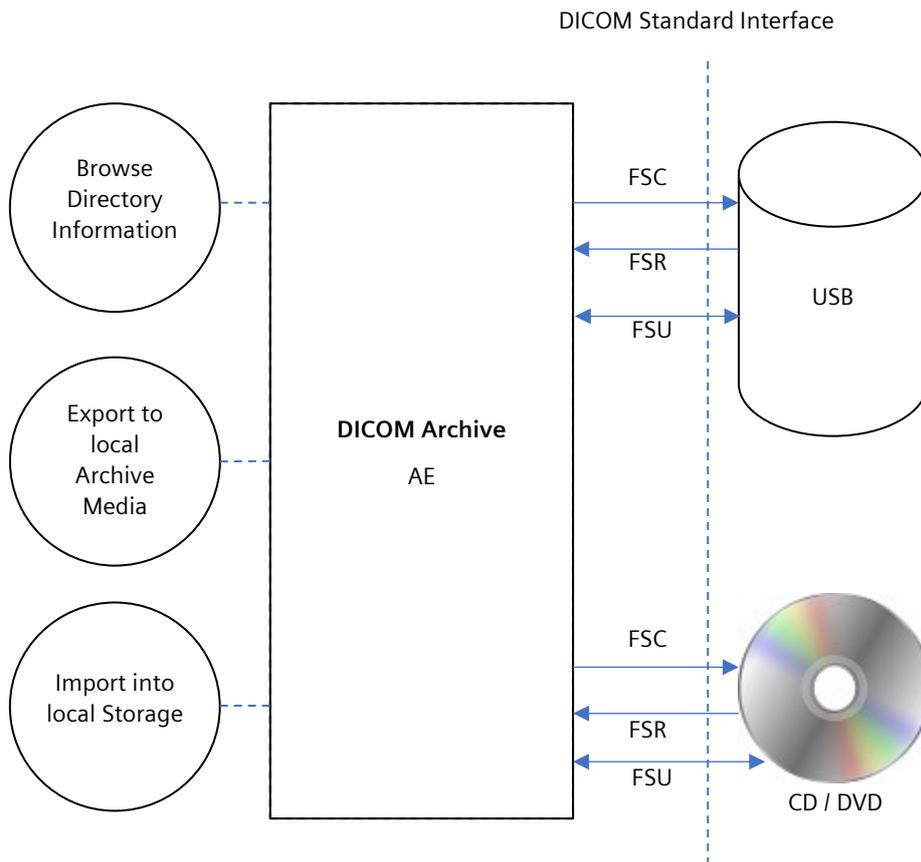
**Figure 8: Media Interchange Application Data Flow Diagram**
