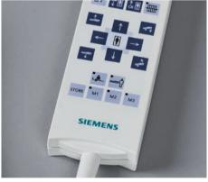
Uroskop Omnia's hand-held control features large intuitive symbols for remote operation of all system and imaging functions
