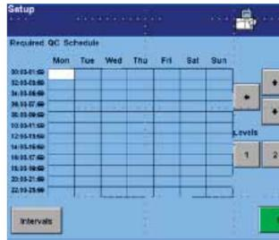
Figure 3. Siemens blood gas analyzers can be configured to meet user-defined QC schedules. Fully customizable QC schedules include selecting the day, time interval and level of QC.
