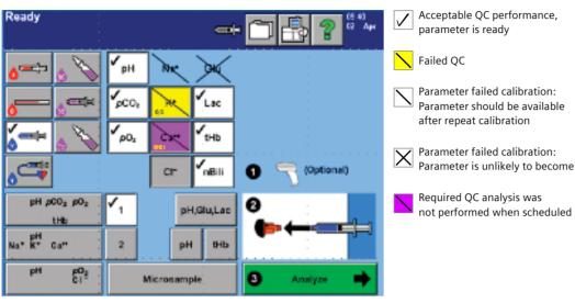
Figure 2. Siemens RAPIDLab 1200 and RAPIDPoint 400 Series analyzers automatically report acceptable and unacceptable QC results for multiple analytes
