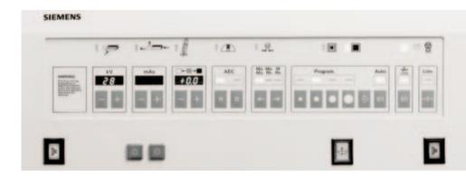
Both Siemens MAMMOMAT 1000 and Siemens MAMMOMAT 3000 Nova are equipped with automatic exposure control (AEC).
