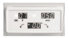
When using Opcomp: Begin by applying compression until the compression plate comes into contact with the skin (3-5 kg). Smooth out any folds in the skin.
