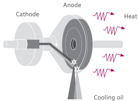
STRATON X-ray tube with z-Sharp generating two distinct X-ray projections.
