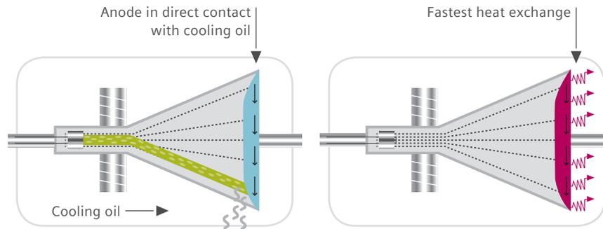
STRATON tube design. The backside of the anode can be cooled directly. Therefore, large heat storage capacity is not necessary, which allows for a very compact design.
