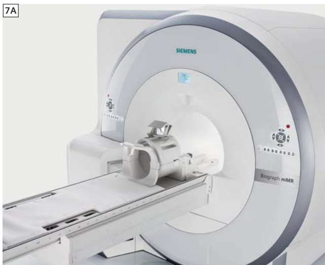
7A (A) A head/neck RF coil that was designed and optimized towards PET-transparency for use in simultaneous MR/PET hybrid imaging. This RF coil serves as an example of a rigid hardware component that is stationary at its known position with regard to the patient table. (B) 3D CT-scan of this rigid RF coil. Such a CT-scan provides hardware attenuation values that can be transformed from the CT's 100 keV energy level to the 511 keV energy level of PET in order to derive a PET-equivalent attenuation map ( \mu -map), shown in image (C). The \mu -map in (C) has been acquired at level a-b as shown in image (B).
