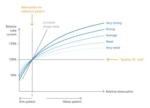
The measured values from the topogram are compared to the built-in reference value yielding a relative attenuation (x-axis). Based on the selected CARE Dose4D curve the relative change of the "Quality reference mAs" is determined (y-axis).
