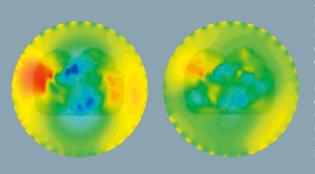
TimTX TrueForm technology enables uniform RF distribution in all body regions. It is a robust method for B1 homogenization, supporting excellent image quality and diagnostic confidence.
