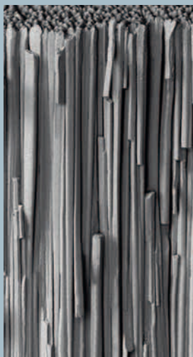
Solid Screen (CsI is grown in needles)
