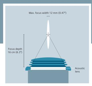
A dedicated design of the shockwave head including the acoustic lens ensures an optimized energy distribution in the target volume.
