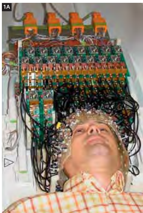
1 Graham Wiggins, one of the authors, tests the 90-channel 1.5T brain array prototype (left) and the 96-channel 3T array prototype (right). The system is a prototype 128-channel MAGNETOM Trio, A Tim System.
