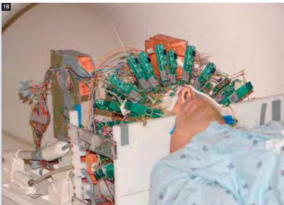
1 Graham Wiggins, one of the authors, tests the 90-channel 1.5T brain array prototype (left) and the 96-channel 3T array prototype (right). The system is a prototype 128-channel MAGNETOM Trio, A Tim System.
