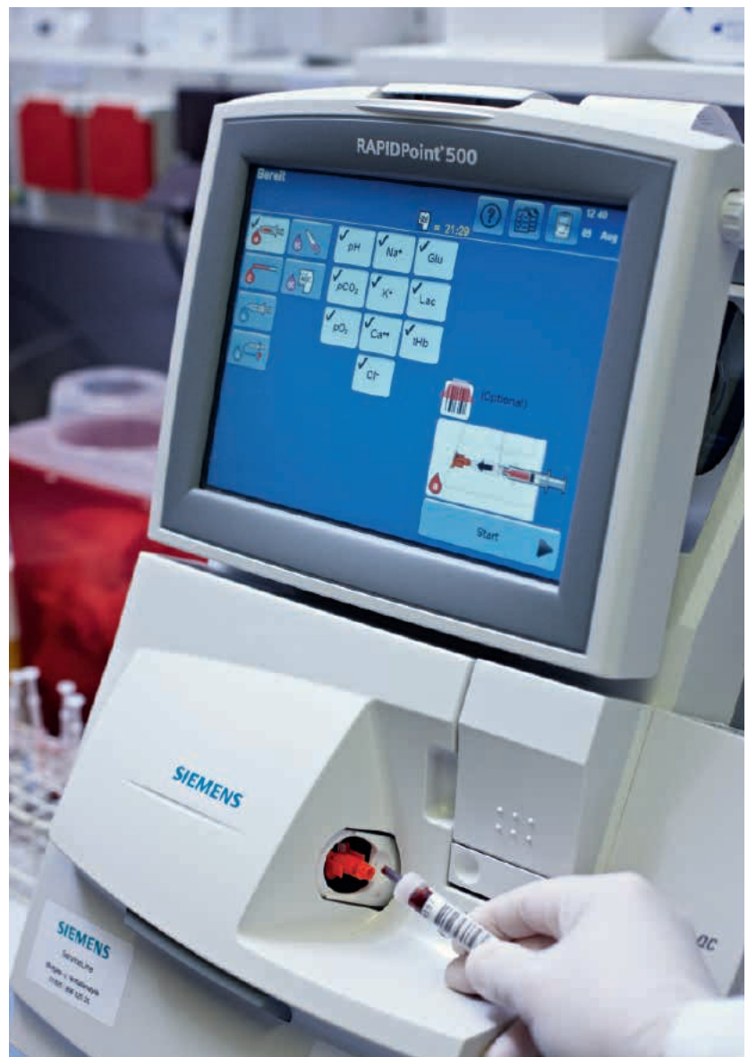
The RAPIDPoint 500 blood gas system determines a patient's full parameter panel, including lactate, in approximately 60 seconds.
