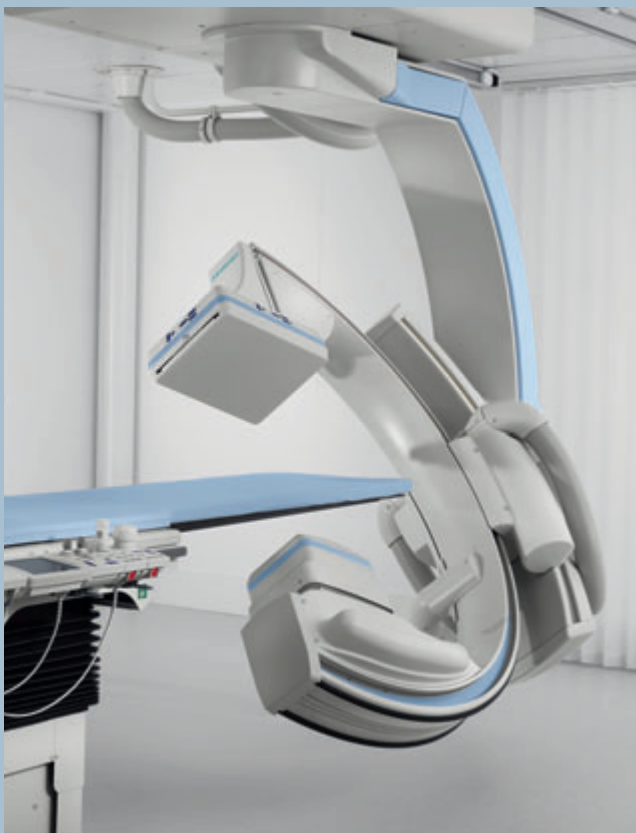
The Artis zee ceiling-mounted system features a 20 x 20 or 30 x 40 flat detector and enables flexible positioning around the patient.
