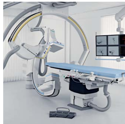
Artis zee biplane The biplane system offers excellent coverage and flexibility for the complete applications spectrum, including neuro, spine as well as pediatric imaging during surgery.
