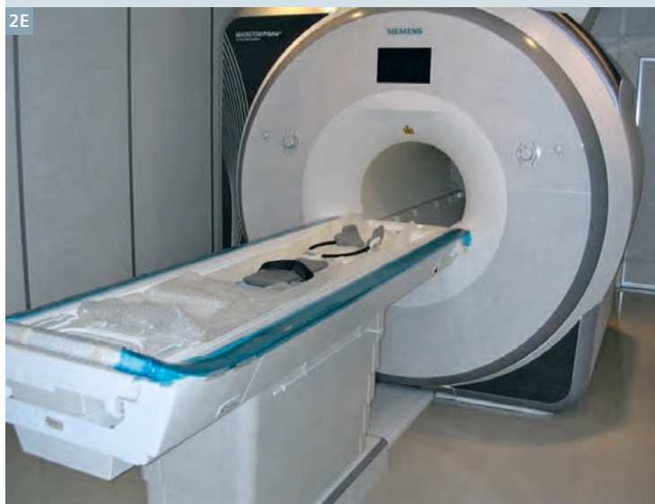
2 These images show the building steps during the fit-upgrade of the MAGNEOM Trio a Tim System (2A). After removing all the old system components (2B) the installation of the new Prisma fit components was carried out by introducing the new gradients (2C) the new Tim covers (2D) and examination table (2E).
