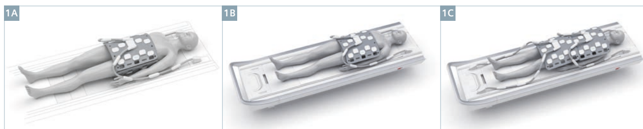
1 The Body 60 coil is designed to serve a broad range of clinical applications. (1A) 'Sandwich' mode, i.e. for pelvic, abdominal or lung exams. (1B) Individual operation as a single Body 30 coil, also possible with 48-channel systems. (1C) Whole-body setup, in combination with the integrated 32ch Spine coil and a 20ch Head coil (not shown here).
