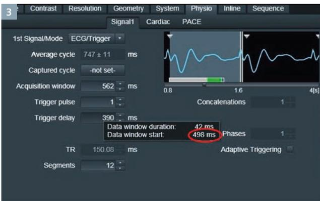
3 The trigger delay is selected, such that the data window start matches the onset of the quiescent period previously identified.
