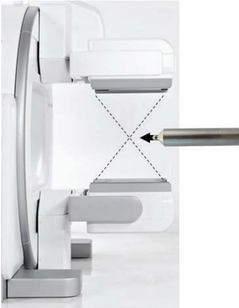
Figure 28: CSS is inserted into Symbia Intevo and supported by the integrated source holder (not shown). The dashed lines depict the FOV.
