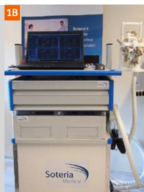
Figure 1: The RCM-system. (1A) MRI-compatible robotic device that holds and manipulates the position of the needle guide. (1B) Cart that is positioned outside of the MRI-room and connected to the robotic device by plastic tubing, containing a steering unit, compressor and vacuum pump. The system includes a portable laptop with the control and targeting software.
