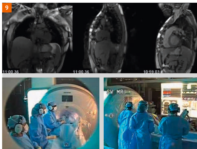
Figure 9: Real-time interventional MRI using the Gadgetron. The top row of images shows example real-time frames used to guide a passive catheter in the patient. The tip of the catheter is equipped with a balloon filled with a Gadolinium based contrast agent. An interactively controlled saturation pulse is used to provide contrast between balloon and surrounding tissue. Bottom row of images shows the interventional cardiologists using the real-time images for navigation.
