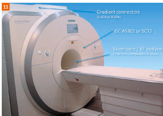
Figure 11: Modified MAGNETOM Skyra system. Dimensions of the RF body coil, patient table and cover were adjusted to the size requirements of both Connectom gradient coils.
