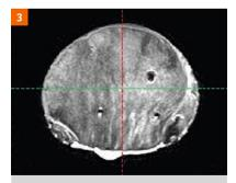
Figure 3: MRI of the pork loin with two markers of 0.5% and one of 2.5% iron content.
