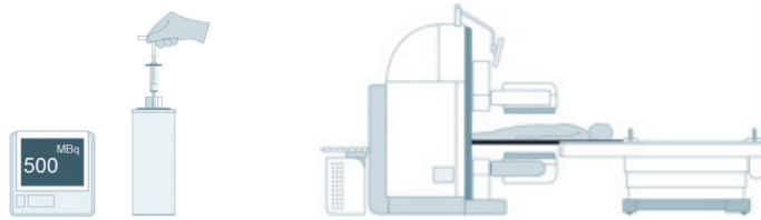
Figure 5b: xSPECT method calibrates the scanner and helps cross-check the dosimeter accuracy using the same calibrated source.
