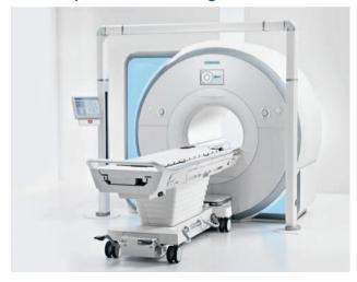
The optional LAP DORADOnova MR3T Laser Bridge is an external laser system supporting virtual simulation at the MR with red or green laser lights. For high accuracy the marked position is shifted to the center of the scanner when using the RT Dot Engine, so there is no need to use the laser of the MR scanner in addition.
