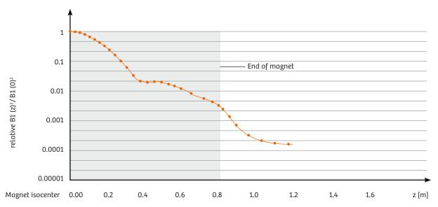
RF power distribution relevant for assessing exposure to MR operators. The diagram shows the RF power distribution along the patient axis of the MAGNETOM Skyra according to the requirements of the IEC 60601-2-33 standard.
