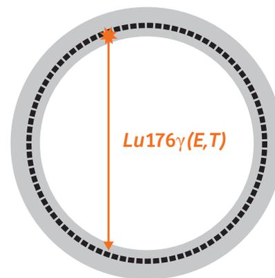
The PET/CT scanner records the position and the time difference of the events from the <sup>176</sup>Lu decay to create a line of response that can be used for scanner setup and quality checks.
