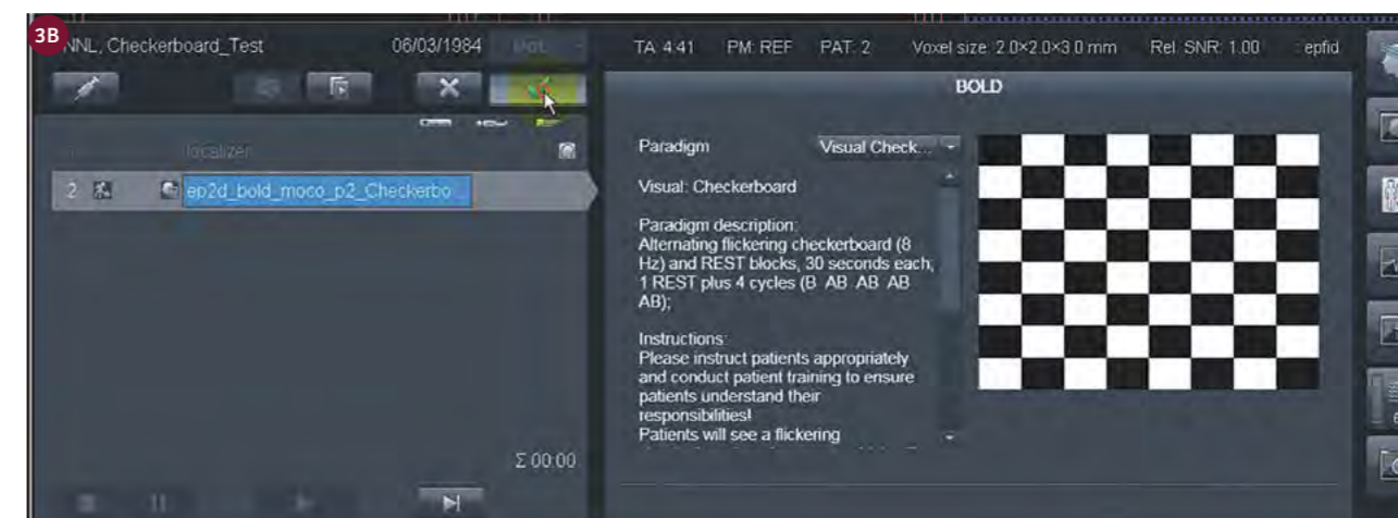
3 When enabling the BOLD Dot AddIn, the user can select the paradigm directly in Siemens Numaris (3A). The lower image (3B) shows that a visual stimulation paradigm has been selected.
