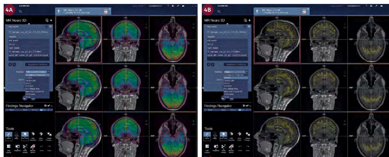
4 Dropdown menu for different overlay palettes in the Control Area on the far left of the screen. These different overlay palettes can aid assessment of co-registration accuracy. The different examples shown are (4A) Advanced Perfusion (default) and (4B) Edges.
