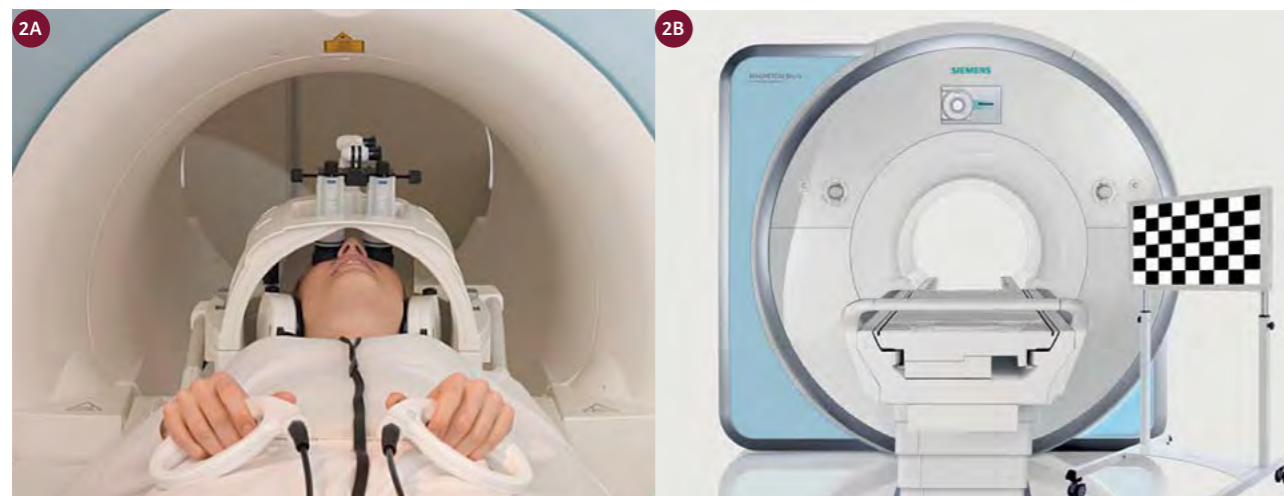
2 The NNL VisualSystem attached to the headcoil (2A), or the NNL InroomViewingDevice (2B) are displaying the paradigm during fMRI. The NNL AudioSystem and ResponseGrip (2A) are used to provide audio stimuli and to collect patient response.
