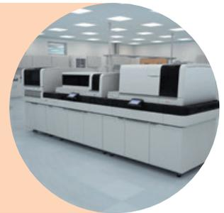
The Atellica™ Sample Handler is the sample processing component of the Atellica Solution and serves as the input/output interface regardless of the number of connected analyzers. The patented Atellica Magline™ Transport connects all components in an integrated workflow. A multi-camera vision system with 360° view is designed to reduce bar-code reading errors, exception handling, and operator intervention.
