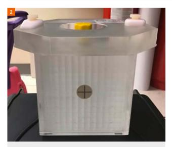
Figure 2: Quasar GRID<sup>3D</sup> image distortion phantom: "small phantom".
