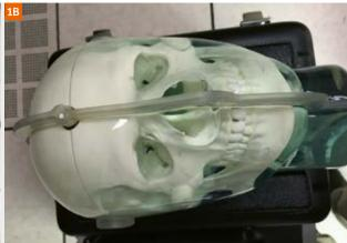
Figure 1: CIRS Simulated MRI distortion head phantom.
