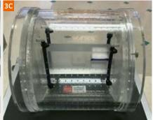
**Figure 3:** Quasar MRID<sup>3D</sup> geometrical distortion phantom: "big phantom".
