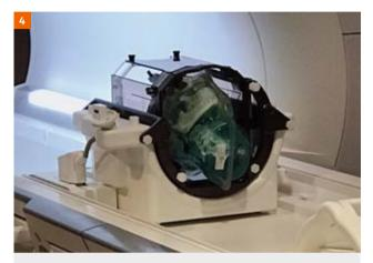
**Figure 4:** CIRS head phantom with SRS frame and all localizer devices.
