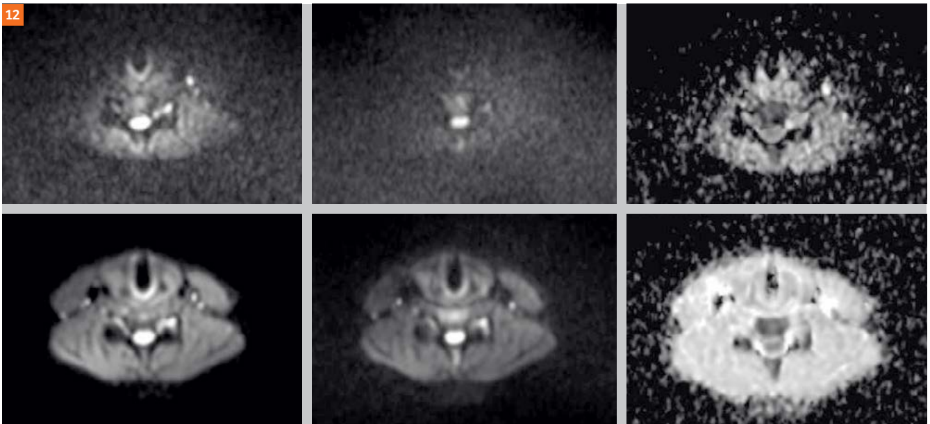
Figure 12: Combining CoilShim with SliceAdjust leads to significant image quality improvements in diffusion-weighted imaging. The same slice is compared without CoilShim and SliceAdjust (upper row) and with active CoilShim and SliceAdjust (lower row). From left to right: b=50 \text{ s/mm}^2 , b=800 \text{ s/mm}^2 , ADC.
