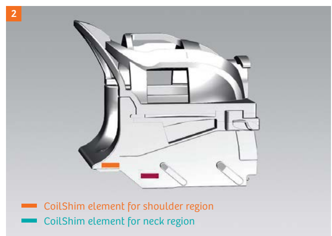
Figure 2: BioMatrix Head/Neck 20 TCS coil design and the location of the CoilShim elements in the BioMatrix Head/Neck 20 TCS coil.
