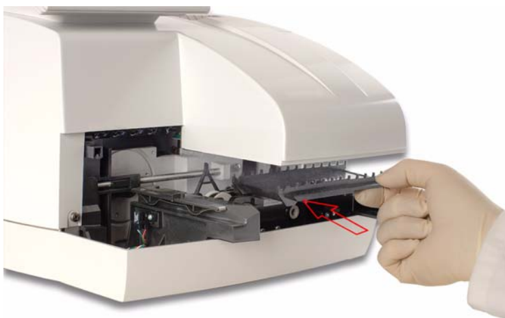
Figure 8-4: Install the Moving Table
