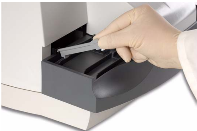
Figure 8-7: Install the Push Bar
