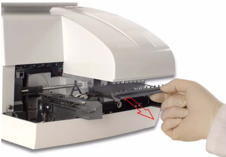
Figure 5-3: Remove the Moving Table
