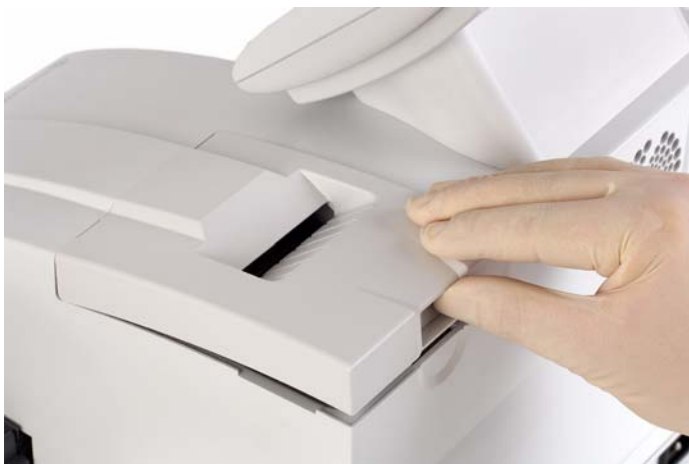
Figure 5-5: Remove the Printer Cover
