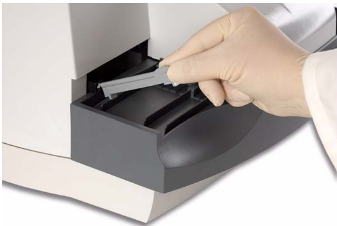
Figure 5-1: Remove the Push Bar
