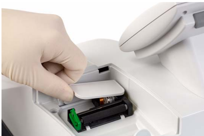
Figure 5-10: Remove the Printer Shield
