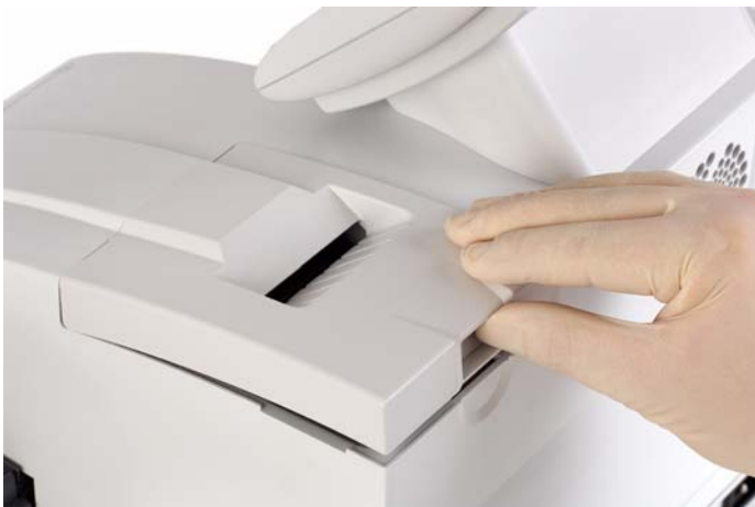
Figure 5-8: Remove the Printer Cover
