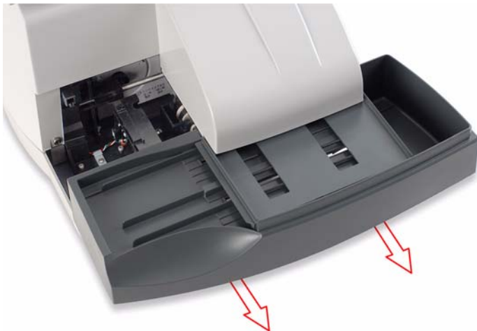
Figure 5-2: Remove the Fixed Platform
