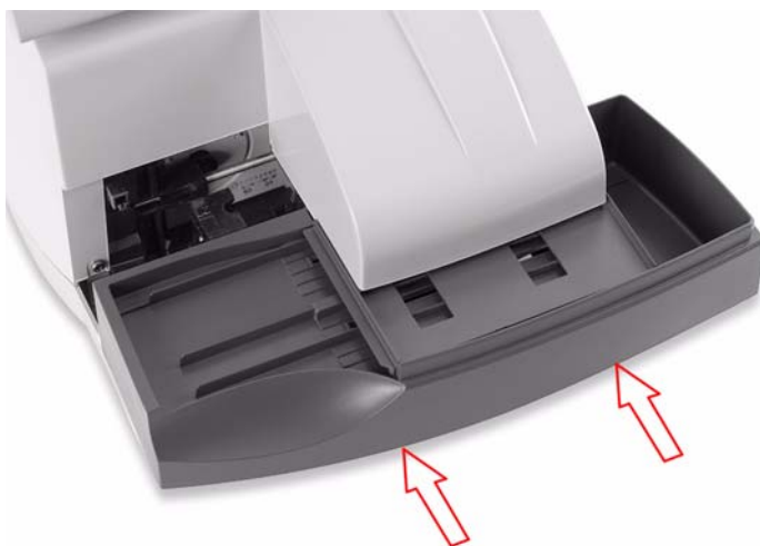
Figure 8-6: Install the Fixed Platform
