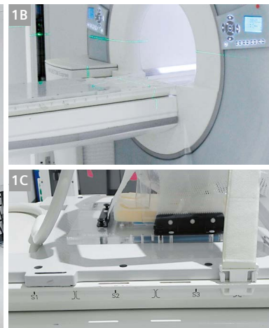
1 (1A) Medibord RT flat couch top (1B) access to head coil fixtures (1C) retaining access to coil securing fixtures and utilizing these fixtures for securing the couch top in position.
