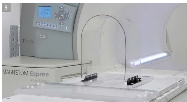
3 In-house manufactured coils support for brain and head and neck imaging.
