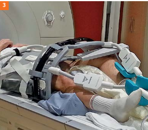
Figure 3: MR Sim setup for TimCT of femur using a combination of coils including 18-channel surface coils and two 4-channel flex coils.
