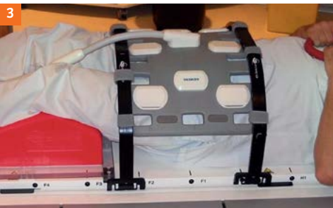
Figure 3: Coil positioning with Body 18 Long coil. The coil holders prevent the coil from pressing on the skin contour. The knee support sits on a moveable rail created at the workshop. The knee support should be the same type as in CT to obtain the best reproducible patient positioning.
