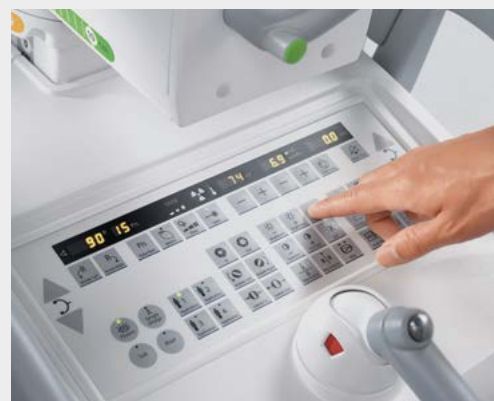
The intuitive button-based user interface facilitates system operation and is easy to clean.
