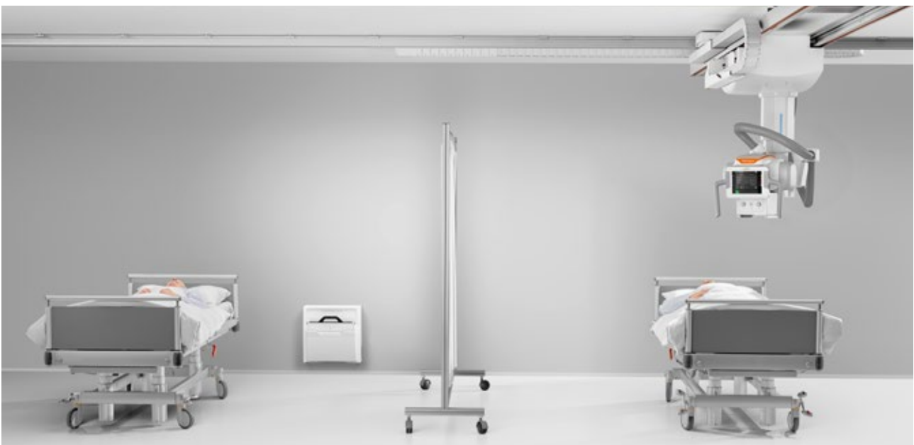
Covers up to 8.5 m in trauma bays with AIM Plus high-speed automation
