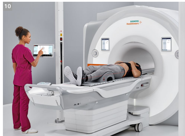
10 MAGNETOM RT Pro edition with external laser bridge from LAP, showing the laser markings on the patient
