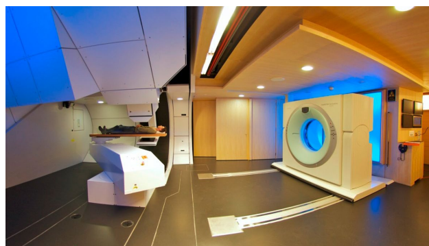
Figure 5. Gantry 2 at PSI showing the treatment machine (left) and the CT sliding gantry (right) used for daily positioning and adaptive therapy
