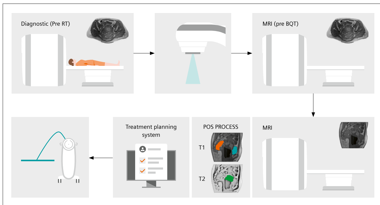
3 IGABT workflow using syngo.via RT post-processing software. RT = radiotherapy; BQT = brachytherapy; POS PROCESS = post-processing.
