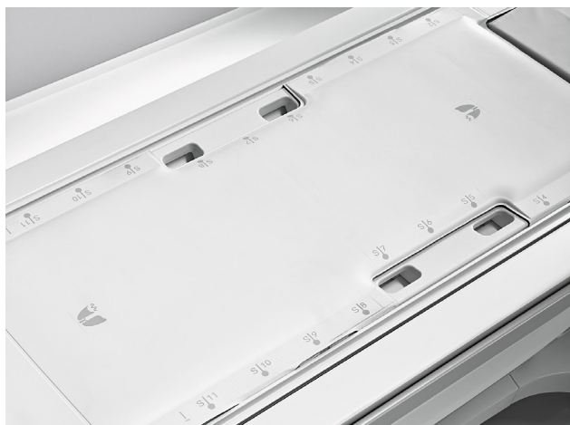
6 The location of the two transmit/receive coils used for respiratory sensing are indicated on the surface of the patient table/spine coil by the lung icons (at the top and bottom). The patient can be positioned head or feet first, with the diaphragm thus lying close to one of these two coils, for detection of respiration.
