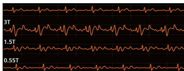
2 The native ECG signal (top row), is barely distorted at 0.55T, whereas distortions become stronger with increasing magnetic field strengths (1.5T and 3T).
