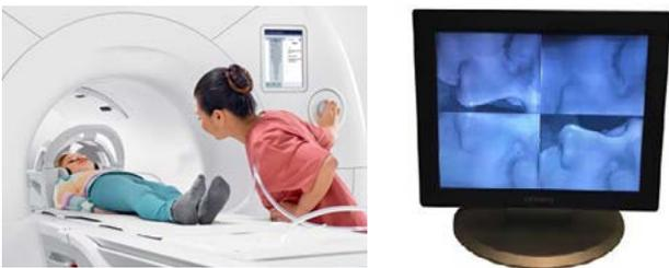
The Kinetic Sensor enables the operator to visually monitor head movement during head exams. The hardware consists of four cameras with a slim profile mounted inside the bore and a monitor to view the patient.
