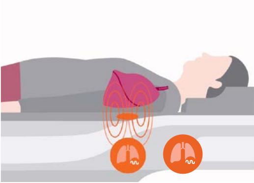
Integrated Respiratory Sensors automatically detect breathing patterns as soon as the patient lies on the table. Respiratory-triggered scans can be performed without additional user interaction to help simplify workflow.
