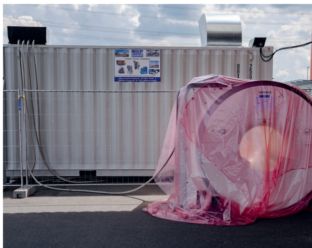
1 Container compressor facility to retrieve helium from old MRI systems that undergo refurbishing.
