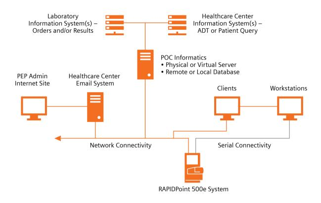
The server requires no static IP addresses but may be configured in static IP address mode if desired by the facility. The following ports are used by the system:
