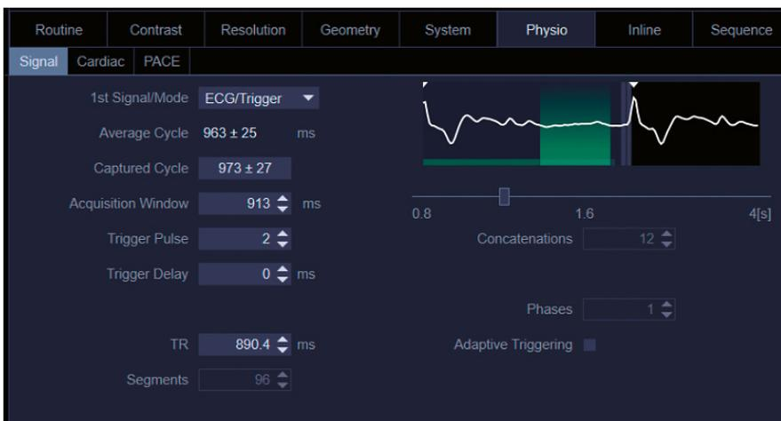
3 Screenshot of the physio signal window on a 1.5T MAGNETOM Sola. The green column in the heartbeat shows the optimal data acquisition time for an LGE sequence.
