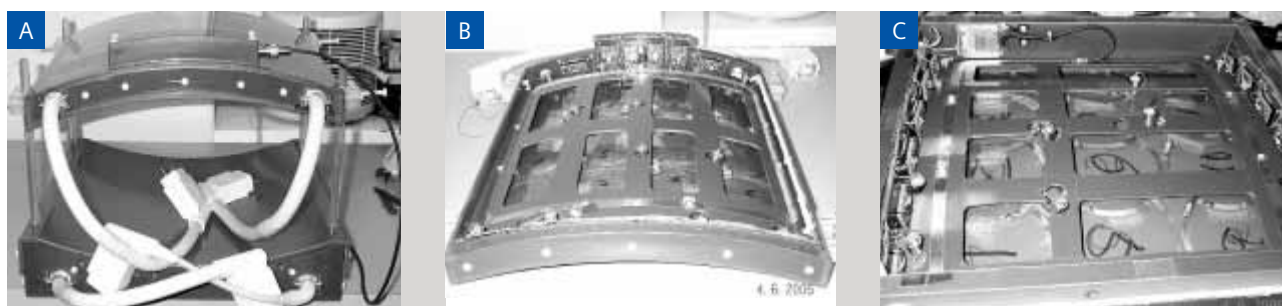
[ Figure 5 ] The appearance of the 2-channel transmit / 24-channel receive phased array system. (A) Is the external view of overall mechanical fixture; (B) top shell internal views; (C) bottom shell internal views
