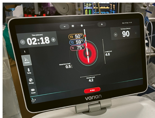
Real-time procedural feedback from temperature sensors as shown on the IntelliBlate System interface
