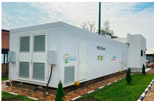
3 A 0.55T MAGNETOM Free.Max with DryCool technology. The system is installed in a mobile unit at the University Teaching Hospital of Kigali, Rwanda.
