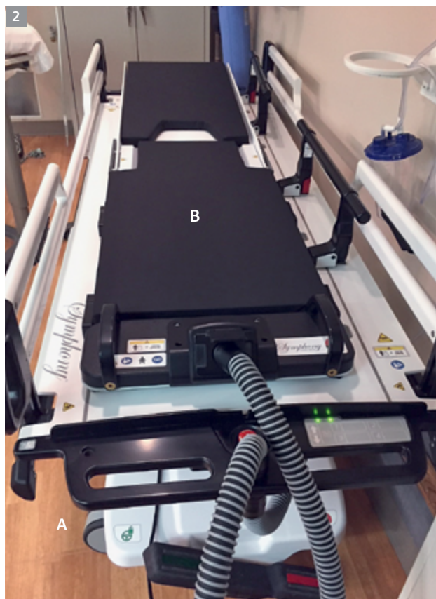
2 Example of a patient transport system (Symphony Patient Transport System, Qfix, Avondale, PA, USA) that can easily move the patient from our Siemens Healthineers Tim Dockable table for the MAGNETOM Aera 1.5T scanner with minimal motion of applicator or needles. (A) Symphony patient trolley-integrated air pump, two batteries, and adjustable pillars. (B) Symphony Brachytherapy Transfer Device and leg extension. All devices are MR Conditional.
