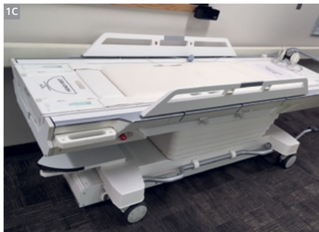
1C The Tim Dockable table detached from the Siemens Healthineers MRI simulator.
