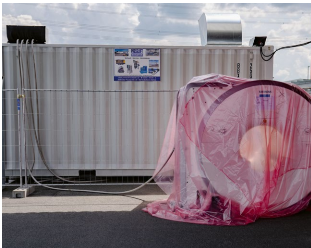
1 Container compressor facility to retrieve helium from old MRI systems that undergo refurbishing.
