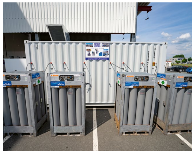
4 Highly compressed recycling helium is filled into gas bottles and returned to gas vendors.
