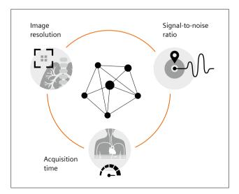
1 Image resolution, SNR, and acquisition time are the three limiting factors of MRI. Using conventional methods, changing one of them directly affects at least one of the two others. Deep learning reconstruction has the potential to disrupt this convention.
