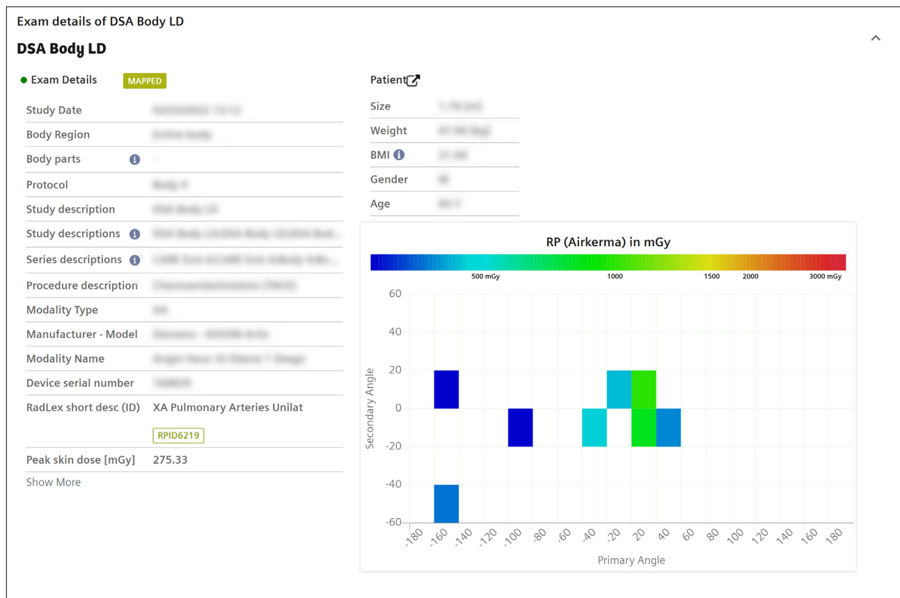
Figure 4: The skin dose distribution view visualizes dose at reference point based on primary and secondary angle. If orange or red pixels appear on the map, the dose is medium or high, depending on the severity of skin reactions it may potentially cause. Skin reactions typically occur after a certain radiation dose threshold.
